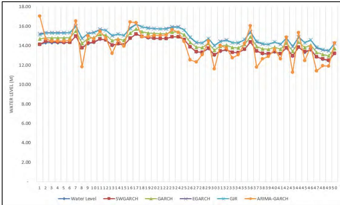
Figure 4.16. Actual and forecast water level for Kuala Nerang station
