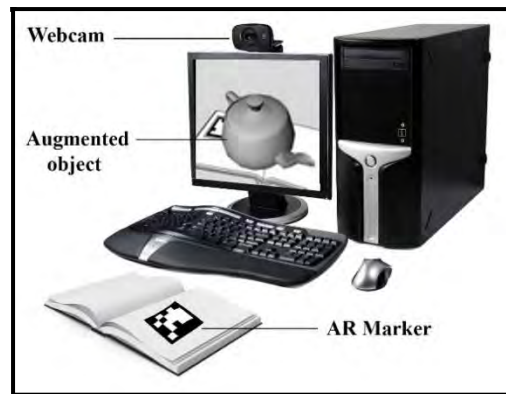
Figure 2.6. Image-based marker AR
