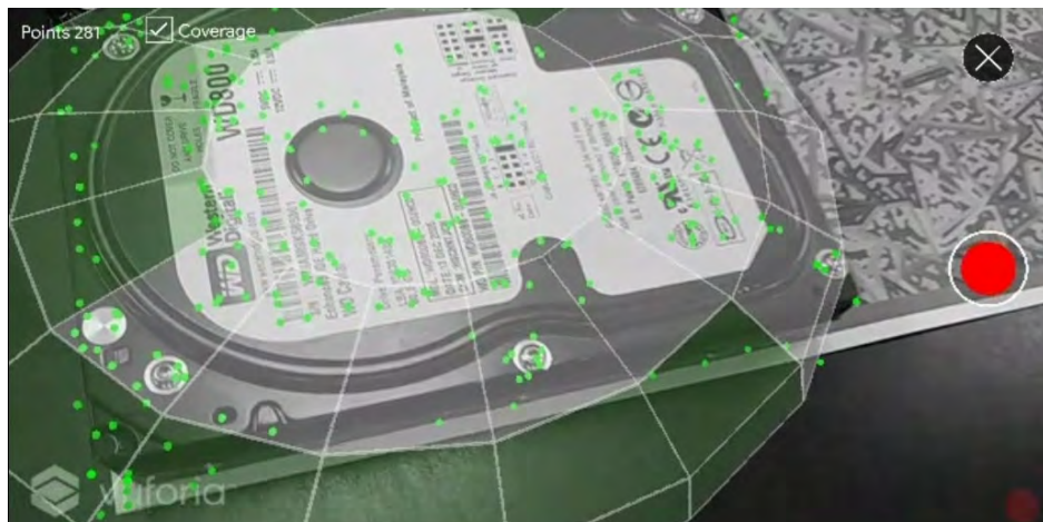
Figure 4.18 : Point scanning process to generate a realistic texture for computer component
