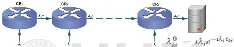
Figure 5.4. Non-coordinated Cache in Series
